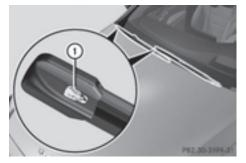
Remove protective film (1) of the service indicator on the tip of the wiper blade.
