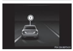
If a lane-correcting brake application occurs, display (1) appears in the multifunction display. The brake application also slightly reduces vehicle speed.
