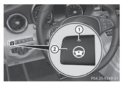
Press button (2). Indicator lamp (1) lights up. The DTR+: Steering Assist. On message appears in the multifunction display. Steering Assist and Stop&Go Pilot are activated.
