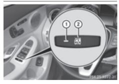
► To activate/deactivate: press button ②. If indicator lamp ① is lit, operation of the rear side windows is disabled. Operation is only possible using the switches in the driver's door. If indicator lamp ① is off, operation is possible using the switches in the rear compartment.
