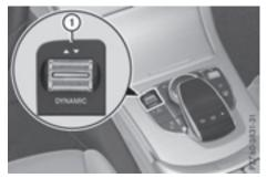
Press DYNAMIC SELECT switch (1) forwards or backwards until the desired drive program is selected.
