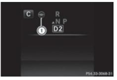
If Steering Assist and Stop&Go Pilot are activated but is not ready for a steering intervention, steering wheel symbol ① appears in gray. If the system provides you with support by means of steering interventions, symbol ① is shown in green.
