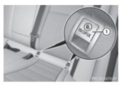
Vehicles with rear seat armrest: adjust the rear seat armrest so that LATCH-type (ISOFIX) securing rings ① for the LATCH-type (ISOFIX) child restraint system are accessible.
