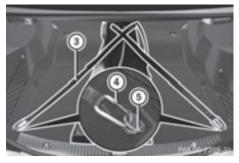
Engage tensioning strap ③ in a diagonal pattern on hooks ④ in cargo tie-down rings ⑤ as shown.
