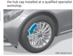
Using lug wrench ③, loosen the bolts on the wheel you wish to change by about one full turn. Do not unscrew the bolts completely.
