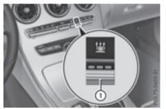
► To activate or deactivate "Immediate preentry climate control": press rocker switch ① up or down. The blue or red indicator lamp above the rocker switch lights up or goes out.
