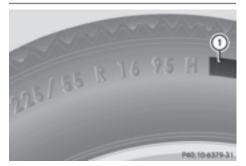
In addition to the load-bearing index, load index () may also be imprinted on the sidewall of the tire. You will find this after the letter that identifies the speed rating ( $\triangleright$  page 374).
