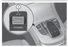
Push DYNAMIC SELECT switch ① forward or back until the desired drive program is selected.
