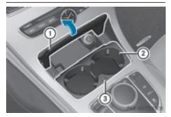
If you remove the cup holder insert, you can use the resulting compartment for stowage.
