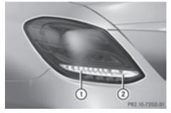
Tail lamp (halogen headlamps) ① Turn signal lamp: PY 21 W
