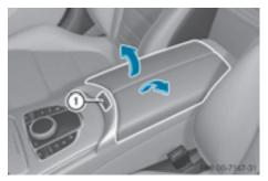
► **To open:** press button ① at the front. The stowage space opens. Depending on the vehicle's equipment, the following may be in the stowage space:
