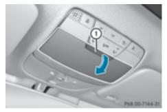
► **To open:** press marking ①. The eyeglasses compartment opens down.
