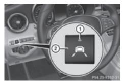
► To activate: press button ②. Indicator lamp ① lights up. The Lane Keeping Assist On message appears in the multifunction display. If all conditions have been satisfied, a warning or steering intervention may be made.
