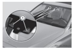
Lane Keeping Assist monitors the area in front of your vehicle by means of multifunction camera ① which is attached behind the top of the windshield. Active Lane Keeping Assist detects lane markings on the road and can warn you before you leave your lane unintentionally. This function is available in the range between 40 mph and 120 mph (60 km/h and 200 km/h).
