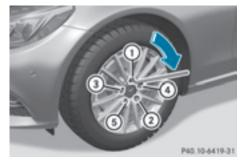
Tighten the wheel bolts evenly in a crosswise pattern in the sequence indicated (1 to 5). The specified tightening torque is **96 lb-ft** (130 Nm).
