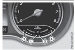
The power display for the electric motor is located on the right-hand side of the instrument cluster.
