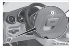
► To apply: push handle ①. When the electric parking brake is applied, the red PARK (USA only) or (②) (Canada only) indicator lamp lights up in the instrument cluster.
