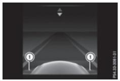
When Active Blind Spot Assist is activated, gray radar waves propagating backwards appear next to the vehicle in the assistance display in the multifunction display. Above a speed of 20 mph (30 km/h), the color of the radar waves in the assistance display changes to green ②. Active Blind Spot Assist is then ready for use.
