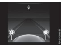
When Blind Spot Assist is activated, gray radar waves propagating backwards appear next to the vehicle in the assistance display in the multifunction display. Above a speed of 20 mph (30 km/h), the color of the radar waves in the assistance display changes to green (1). Blind Spot Assist is then ready for use.
