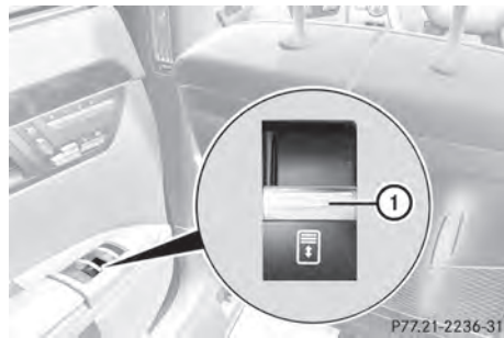
Door control panel in rear
